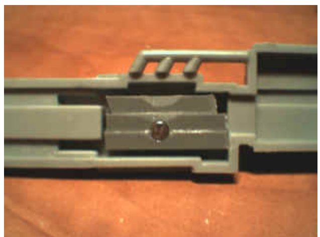
Railgun with embedded magnet.
